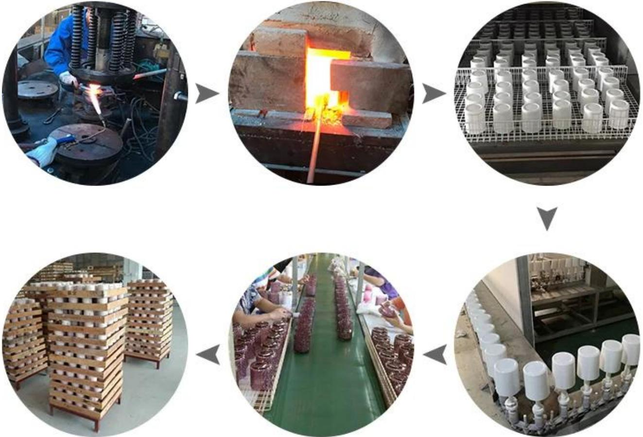
1. The glass is heated in a furnace. 2. The glass is then blown into a mold. 3. The glass is then pressed into a shape. 4. The glass is then annealed in a lehr. 5. The glass is then inspected. 6. The glass is then packaged.
